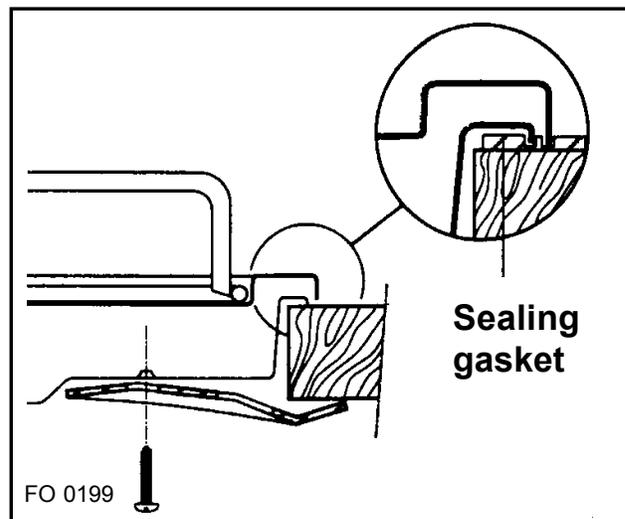
The edge of the hob forms a double seal which prevents the ingress of liquids.
