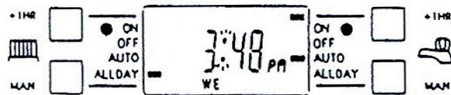
When programming 7 day models, FP75 & CP75, the day being set appears in the display (see typical displays). With 24 hour models, FP15 & CP15, the day only appears in SET TIME mode. When models are being programmed in 5 day/2day mode then the days will show as MOTUWETHFR of SASU. Should the unit be disconnected from the mains a small battery symbol will blink on the left hand side of the display.
